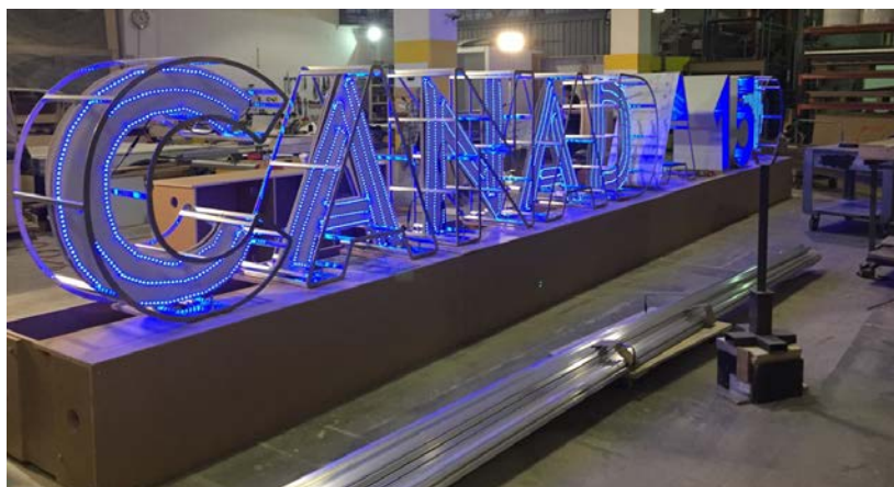
The RoscoLED Tape is tested after being centered inside the CANADA 150 framework
