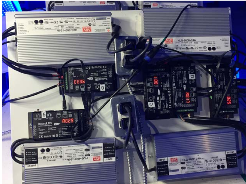
Just a few of the RoscoLED Power Supplies and DMX Decoders used to control the CANADA 150 signs
