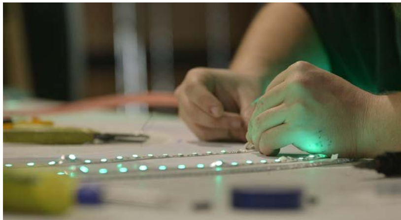
RoscoLED Tape is mounted to Coroplast boards
